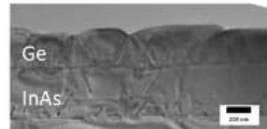
Figure 15: A TEM image of a Ge layer grown on an InAs layer.
